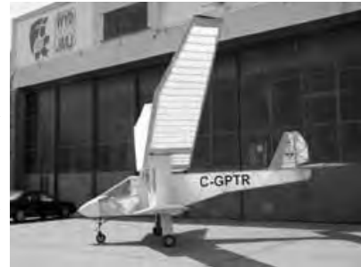
Figure 1. A DeLaurier 2002 flapping wing machine: a synthesis of birds and airplanes.
