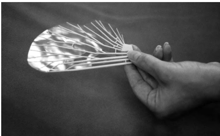
Figure 4. Fused Deposition Modeled wings with interstitial
