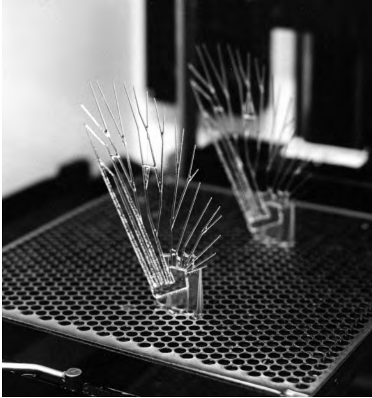
Figure 2. Wings grown using Stereolithography.
