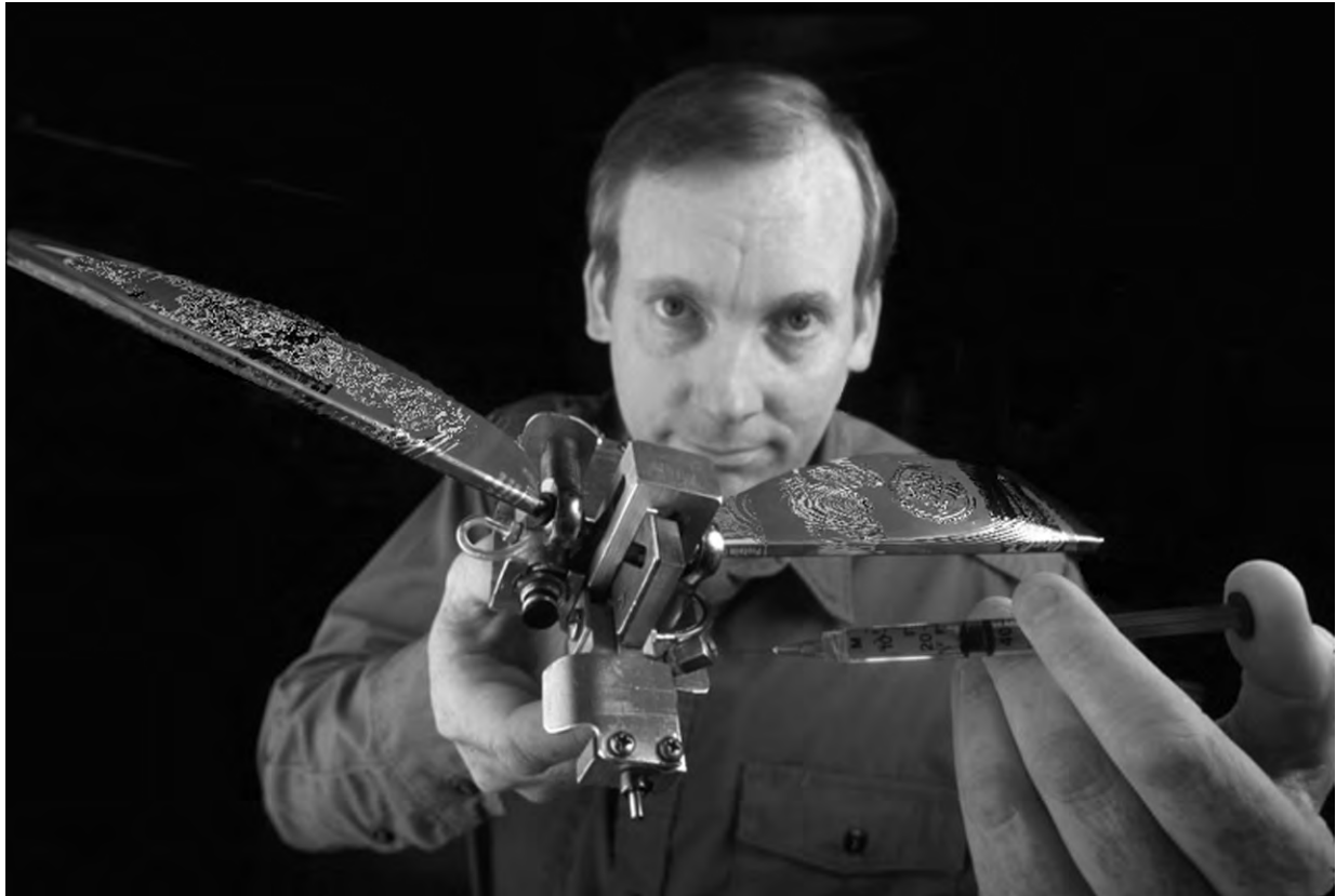
Figure 5. Reciprocating Chemical Muscle Test Bed.
