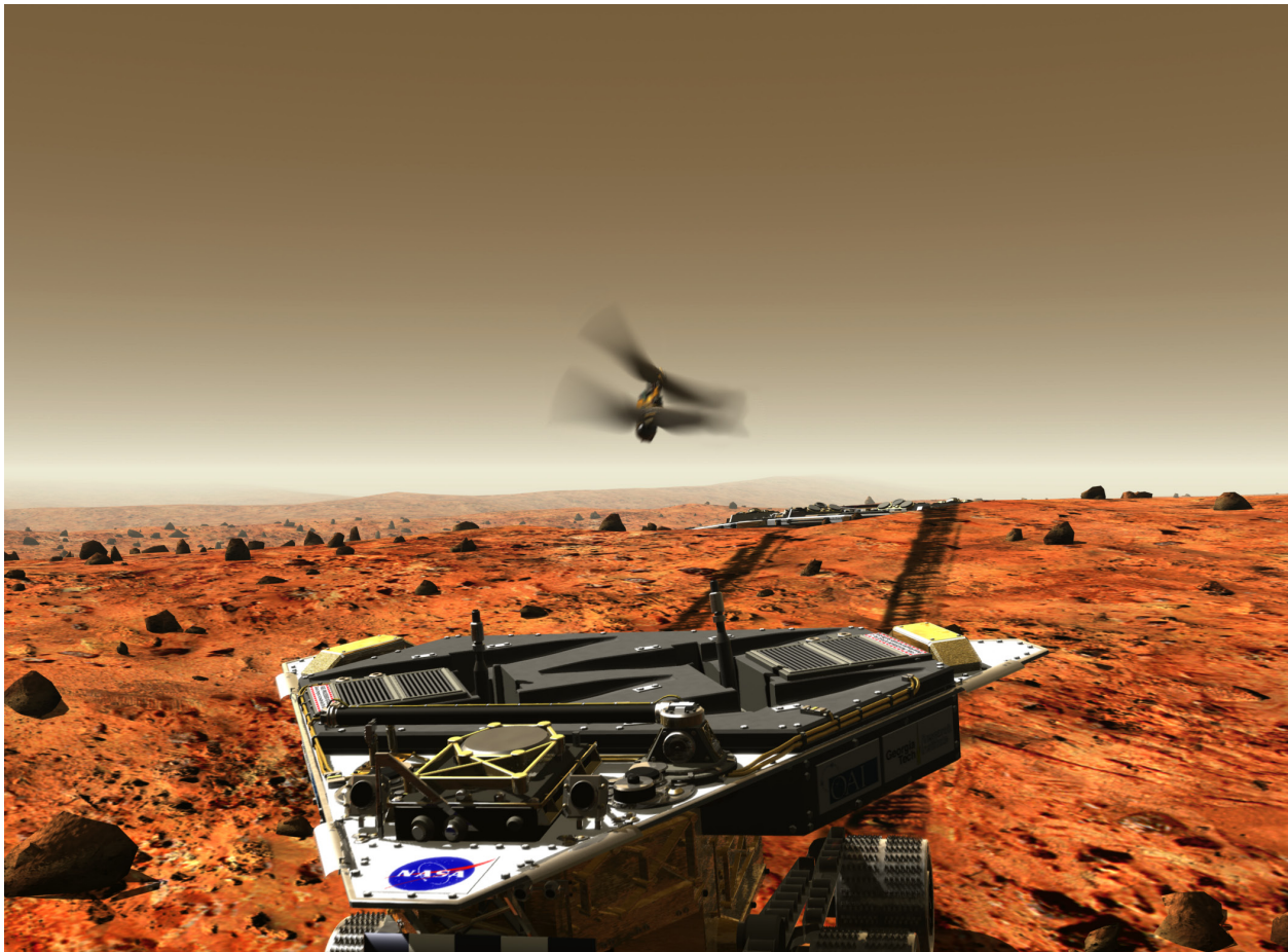
Figure 2. Mars Entomopter operating in the vicinity of its refueling rover.
