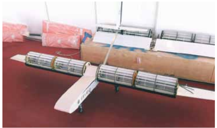
The fan wing, or rolling wing, vehicle from Northwestern Polytechnical University. It is named Hot Wheels.
